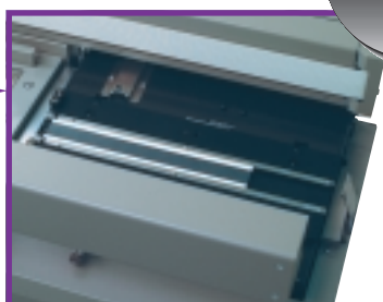
Placing a tape on the nipping station.
