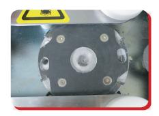
New spine roughening with 1 notching blade and 6 roughing blades provides better glue penetration while applying the glue onto the book spine.
